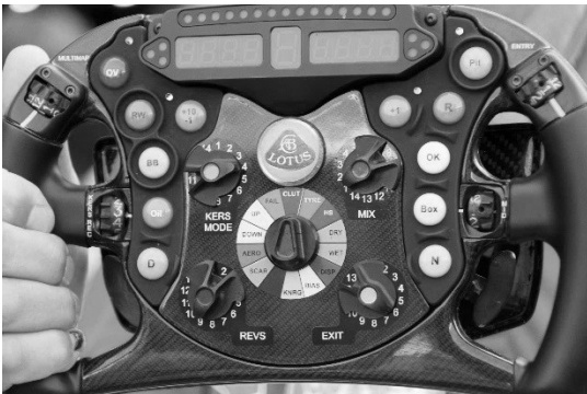
Figure 5: A modern example on an F1 steering wheel with numerous inputs changed. Drivers update the cars setting multiple times per lap depending on conditions.
